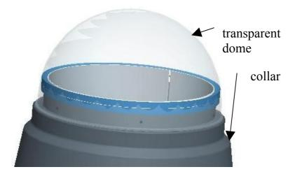
9. Screw the dome using the predrilled holes to the collar in such a way that the screws always pass through the dome, the collar and the tube.
