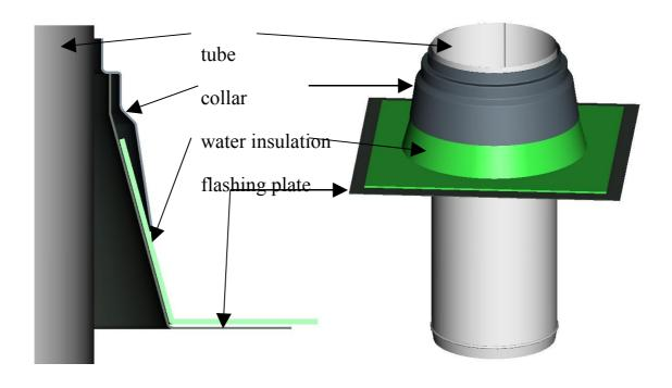
6. Along the circumference of the part of the tube which overlaps the collar, glue one self-adhesive nylon brush seal flush with the tube edge. Glue the other seal to the top edge of the collar. Before you do the gluing, remove any grease from the contact surface. Insert the collar on the flashing plate.
