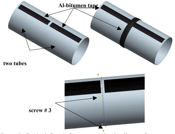
5. Prepare the directional elbows in the same way as the tubes. However, first you must set the elbow by turning the individual segments to the required angle. Then remove the protective foil from the inside. The elbow revolving joints must first be screwed together in three, four or six places (or riveted with a 3 mm stainless steel rivet inserted in a 3.2 mm hole), and again the Al-bitumen tape must be applied over it and heated with the hot air gun.
