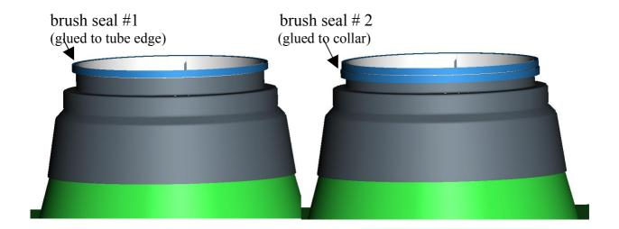
7. As a result of the endeavour to achieve the best possible sealing effect between the tube and the collar, it sometimes happens (within manufacturing tolerances) that the collar is difficult to insert on the tube (overlap). Therefore, in these cases it is necessary to trim part of the lock (the lip) under an acute angle so that the tube diameter fits the collar (see the figure below).
