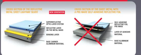
PVD (Physical Vapour Deposition) process in a vac- metal because of the cost cutting which brings uum, during which superreflective and reflection- a high risk of the loss of the adhesion and enhancing layers are applied continuously to the the damage of the mirror surface. base material, is a homogenous, superreflective, flexible, mechanical and chemical resistant surface.
