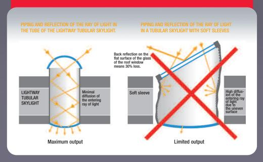
Lightway provides 300% higher brightness than the skylights using soft sleeves for piping light. To illustrate this point the LIGHTWAY the street than skylights with soft sleeves of the diameter 550 mm. The superreflective LIGHTWAY surface has the reflectance of 99,8% and a very low tubular skylight with the diameter 320 mm percentage of diffusion of the ray of light
