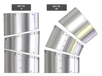
Figure 8 - Adjustment of Elbows
