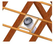
Figure 5 - Use of Auxiliary **Battens**
